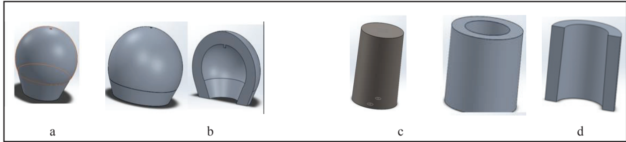
FIGURE 4. Dome feeder (a), dome sleeve (b), cylinders feeder (c) and cylinders sleeve (d)
