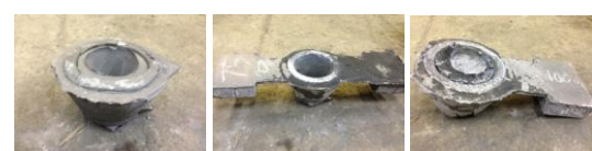
FIGURE 5. bimetallic castings by initial preheating temperature 500 °C(a), 750 °C (b), and 1000 °C (c)
